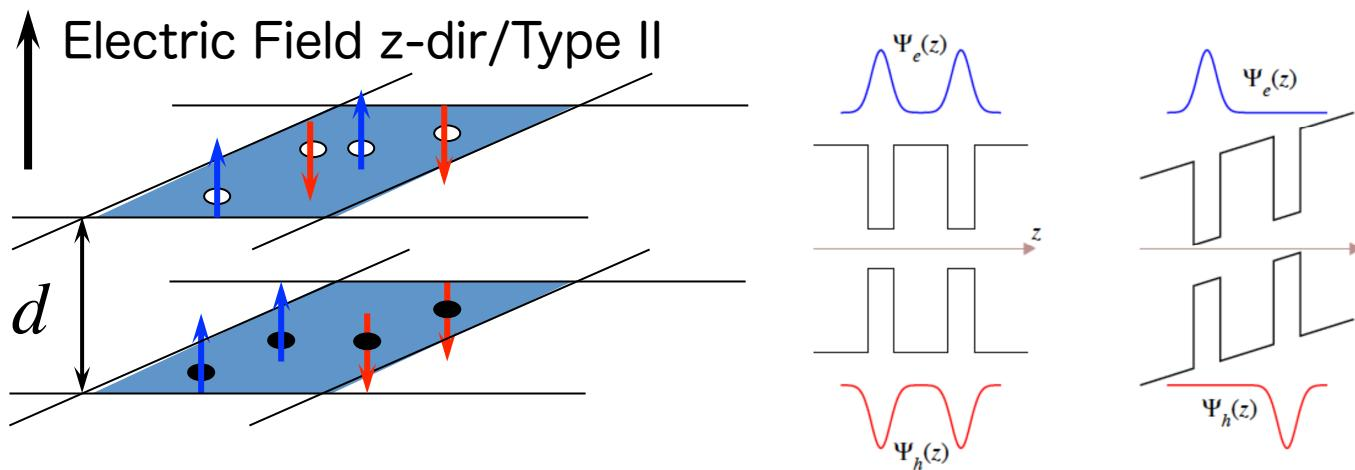
$d \sim 4\text{-}5\text{nm} \sim 100 \text{ a.u.}$  e.g., AlAs/GaAs
