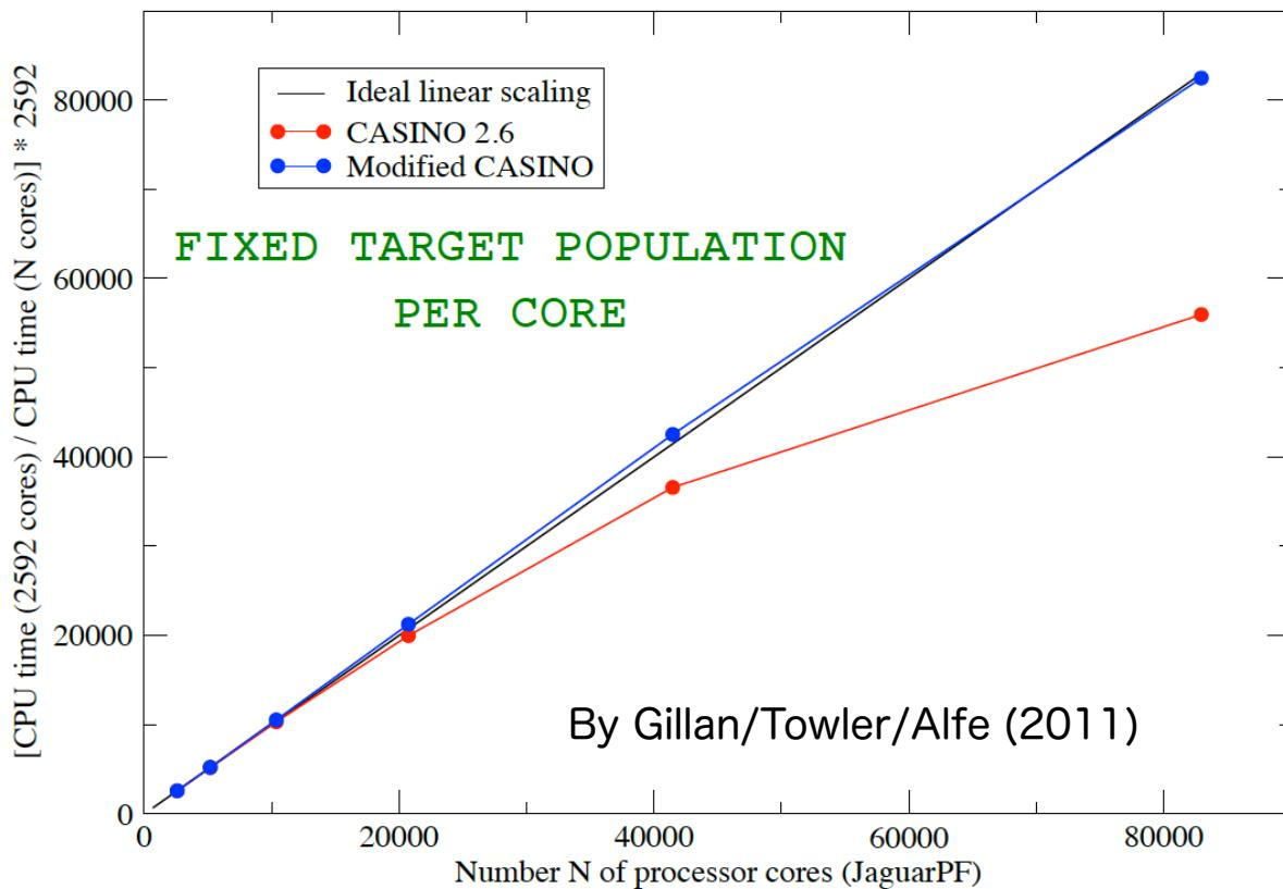
Improved by replacing MPI\_SEND --> MPI\_ISEND
