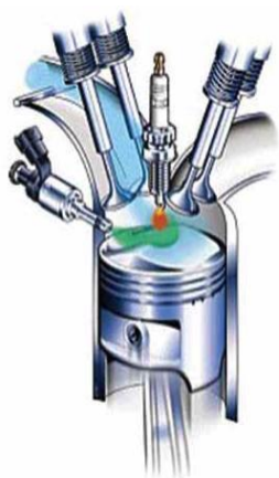
Figure 2: EcoBoost—with direct injection, fuel is injected into each cylinder or an engine in small, precise amounts.
