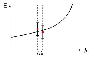
Relative error in finite difference estimate of  $dE/d\lambda$  diverges as  $\Delta\lambda \rightarrow 0$ .
