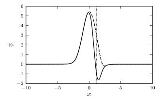
The form of the wave function used for the single electron harmonic well calculations. The dotted line represents the centre of the blip function with coefficient  $\alpha_{14}$ , which is varied between -2.0, giving the solid line, and 2.0, giving the dashed line.
