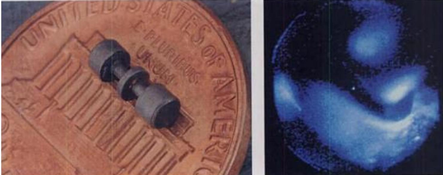
Dehmelt also trapped a single barium atom that he named Astrid, and kept it floating like a pixie in a tiny ion-trap vacuum chamber for ten months. Under suitable conditions, she turned out to be visible to the naked eye..
