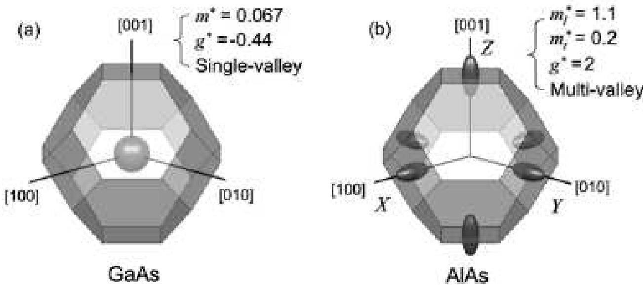
Schematic drawing of the Brillouin zone and constant energy surfaces of the lowest energy bands for bulk GaAs (a) and bulk AlAs (b)
