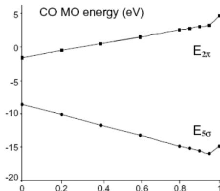
The HOMO and LUMO energies of CO as a function of the amount of exact exchange in a hybrid functional.
