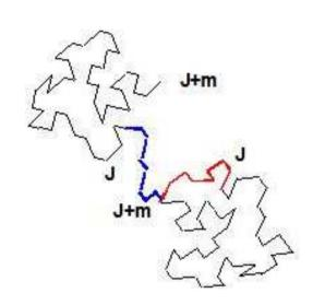
A staging chain is constructed connecting the bead J of atom 1 with the bead J+m of atom 2
