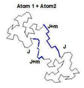
A staging chain is constructed connecting the bead J of atom 2 with the bead J+m of atom 1
