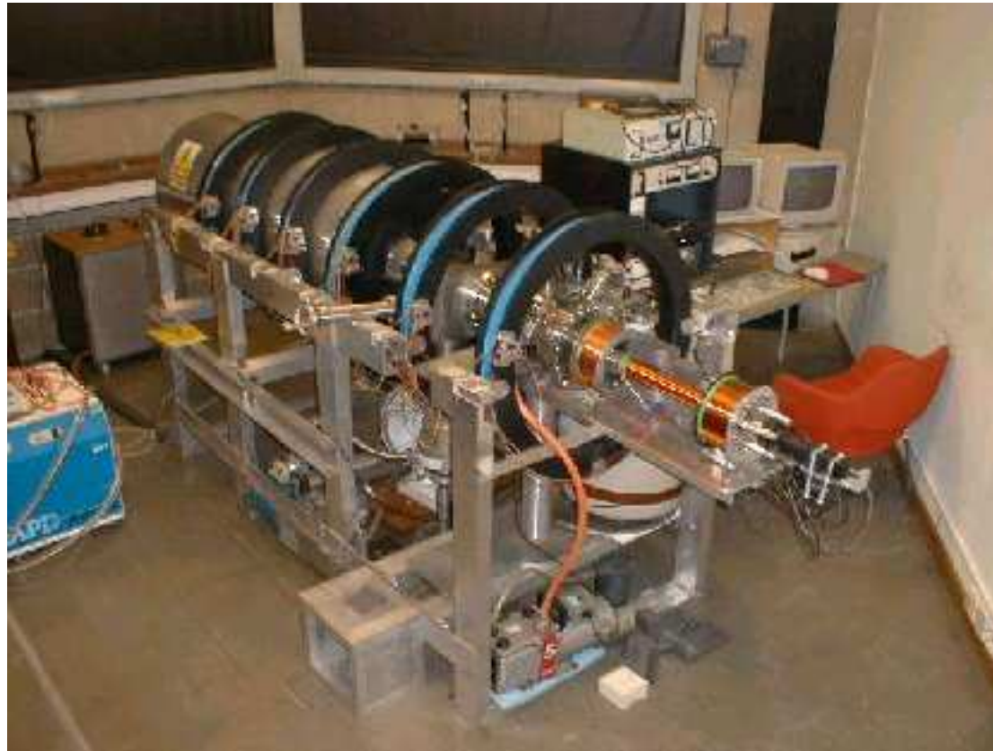
Magnetically confined positron beam for DOBS experiments at the University of Bath
