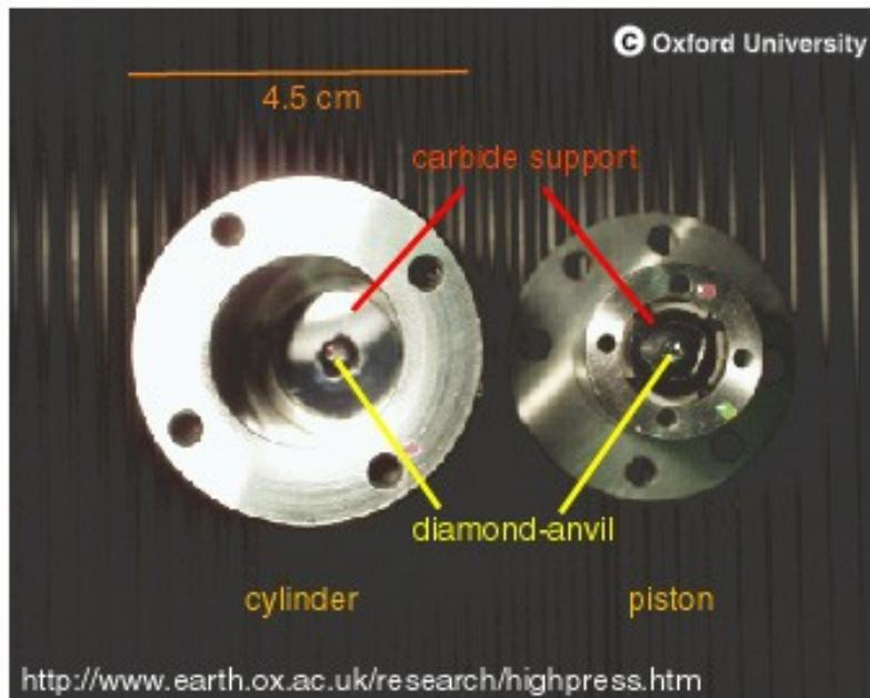
Top view onto an open Mao-Bell type DAC. The main components of the DAC are a long piston-cylinder assembly loaded with a lever arm.
