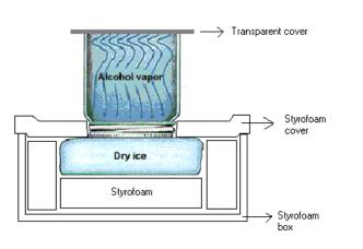
Sealed chamber with supersaturated vapour kept near condensation point by regulating T. Ionizing radiation leaves trail of charged ions that serve as condensation centers. Vapour condenses around them. Radiation *path* thus indicated by tracks of tiny liquid droplets in supersaturated vapour.
